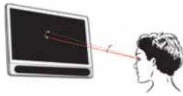
Gaze accuracy and gaze precision are measured in degrees of visual angle. One degree accuracy corresponds to an average error of 11 mm (0.45") on a screen at a distance of 65 cm (26").
